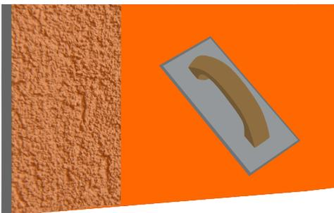
**STEP 6:** Application of **Silblock (Water Repellent Sealer)** over the prepared surface of **Ressi PlastoRend 100**.
