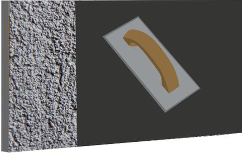
**STEP 4:** Application of **Ressi PlastoRend 100** over the base plastered surface.
