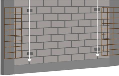
**STEP 2:** Application of **Ressi PlastoRend 120** directly on prepared masonry & Concrete surface.
