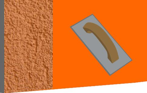
**STEP 4:** Application of **Silblock (Water repellent sealer)** for long term plaster protection.
